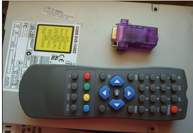
Figure 2: Remote control and IR receiver to be plugged in the serial port
